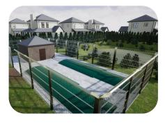
A package te-cyc<sup>™</sup> solution is available to address nitrate and phosphorus concerns for commercial clients and developers. The standard modular units help developers achieve Nitrate Neutrality and come as a complete 'plug and play' system including aeration blowers, chemical dosing and local control panels for automated operation.
