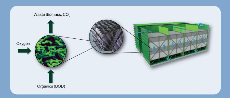
The te-saf<sup>™</sup> is a biological treatment process where specific microorganisms, in a managed aerobic environment, consume biodegradable soluble organic contaminants. An adequate distribution of the organic pollution within the bioreactor increases the probability of contact between colloidal compounds and microorganisms.
