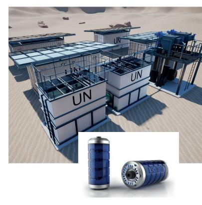
water "inside-out" cycles, will automatically be initiated to clean the clogged group or groups of cartridges whilst the other modules remain in normal operation.
